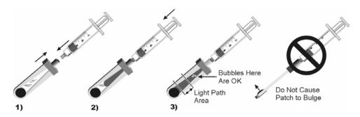
11.4.3.7 Leave the syringe and cuvette attached and insert the cuvette into the test chamber.
