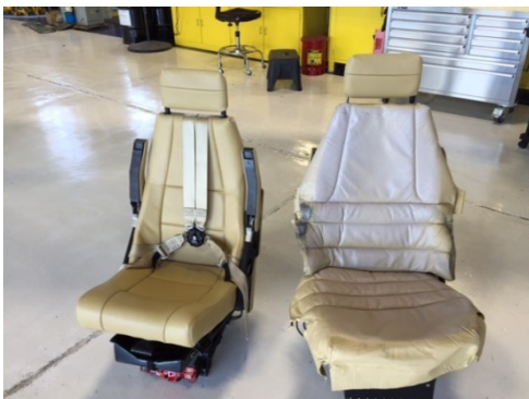
Replaced pilot seat left original seat right.
