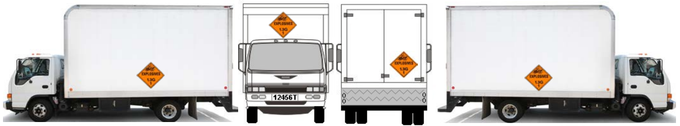
Example: The placard is to be displayed on all sides of the vehicle.
